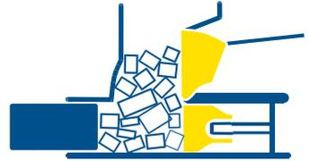
The DH and XH models are equipped with an adjustable feed opening to ensure optimum compression and the correct bale length when baling heavy material. The pressing sequence is the same but the start positions of both prepress and main ram are half way into the press chamber, thus reducing the press chamber volume by 50%.
