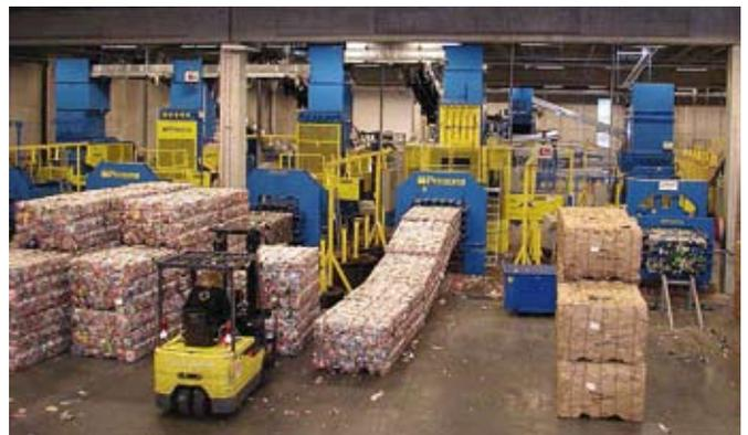
this flow, the plant is equipped with 6 fully automatic balers from Presona in sizes varying from 40 to 100 tons press force. There are also two Presona perforators for mechanical perforation of PET bottles – a guarantee for obtaining maximum bale weight.
