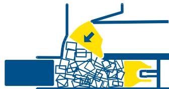
Prepress forces material into press chamber.
