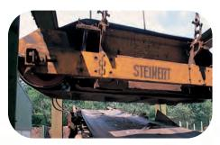
the treatment of slags and pyrolysis coke from thermal refuse treatment. **STEINERT** suspension magnets, mostly permanent magnet models, can be used to process iron-free demolition scrap into a valuable building material. Smaller iron particles, which are not captured by the drum magnet immediately behind the shredder, are extracted from the heavy shredder fraction. Bottle caps and screw tops are removed from collected glass for recycling before it is remelted.
